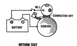
4. Return test:. With a battery connected to the solenoid ter-
