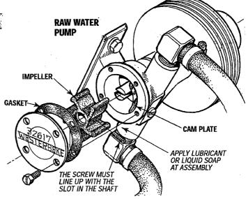
**CAUTION:** If any of the vanes have broken off the impeller, they must be located to prevent blockage in the cooling circuit. They often can be found in the heat exchanger.
