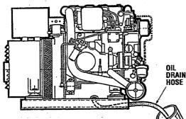
3. Filling the Oil Sump. Add new oil through the oil filler cap on the top of the engine or through the side oil fill. After refilling, run the generator for a few moments while checking the engine's oil pressure. Make sure there is no leakage around the new oil filter or from the oil drain system, and stop the generator. Then check the quantity of oil with the lube oil dipstick. Fill to, but not over the high mark on the dipstick, should the engine require additional oil.
