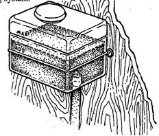
**NOTE:** This tank, with its short run of plastic hose, is best located at or above the level of the engine's exhaust manifold.
