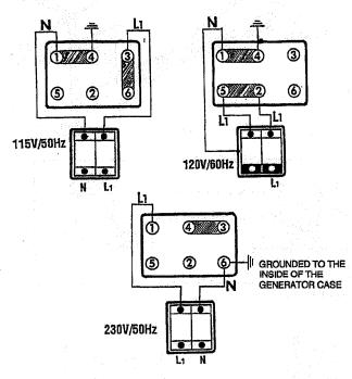
4. Shut off the generator. Make sure the correct Hertz lead (60 Hertz #6, or 50 Hertz #5) is plugged into the capacitor(s).
