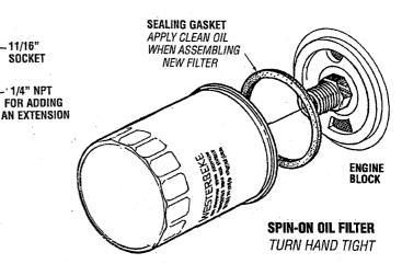
**NOTE:** Generic filters are not recommended, as the material standards or diameters of important items on generic parts might be entirely different from genuine parts. Immediately after an oil filter change and oil fill, run the engine to make sure the oil pressure is normal and that there are no oil leaks around the new oil filter.
