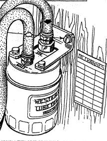
APPLY A THIN COAT OF CLEAN OIL TO THE FILTER GASKET WHEN INSTALLING. AFTER THE FILTER CONTACTS THE BASE, TIGHTEN IT AN ADDITIONAL
