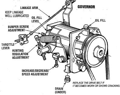
4. Periodically adjust the governor belt tension (see *DRIVE BELT ADJUSTMENTS*). Since belts stretch slightly, this stretching will, to some degree, affect the governor's action.
