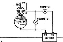
**CAUTION:** Use thick wires as much as possible and tighten every terminal securely. This is a solenoid shifttype starter which makes a rotating sound louder than that of a direct-drive type starter. When detecting starter rotation at the pinion tip, be careful not to come in contact with the pinion gear when it protrudes.
