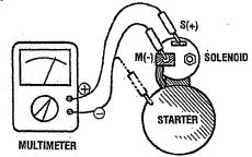
NOTE: Disconnect the wire from terminal M.
